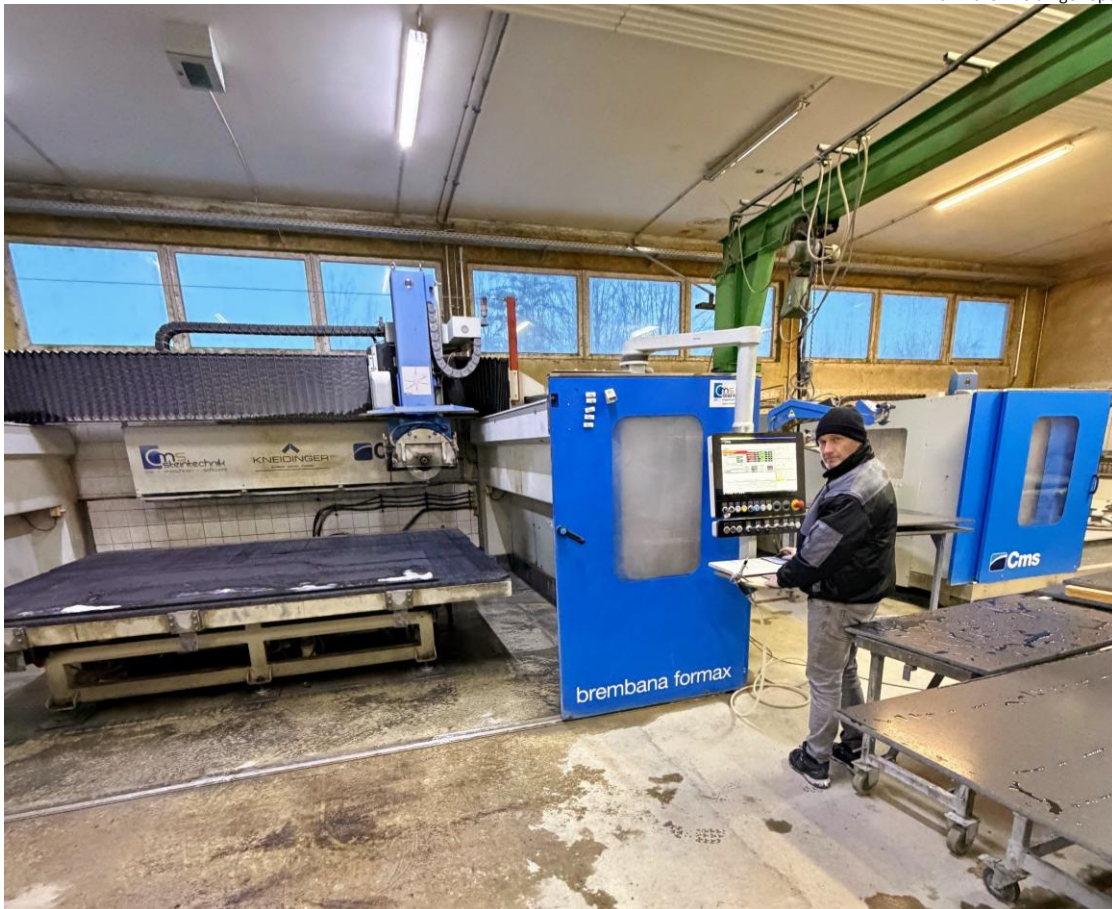
CNC bridge saw and CNC machining centre from CMS digitally linked within the Kneidinger operation
