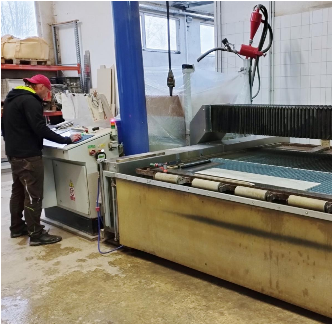
Partially integrated into digital production via TOP / SeCAM V10: the PTV waterjet cutting system
