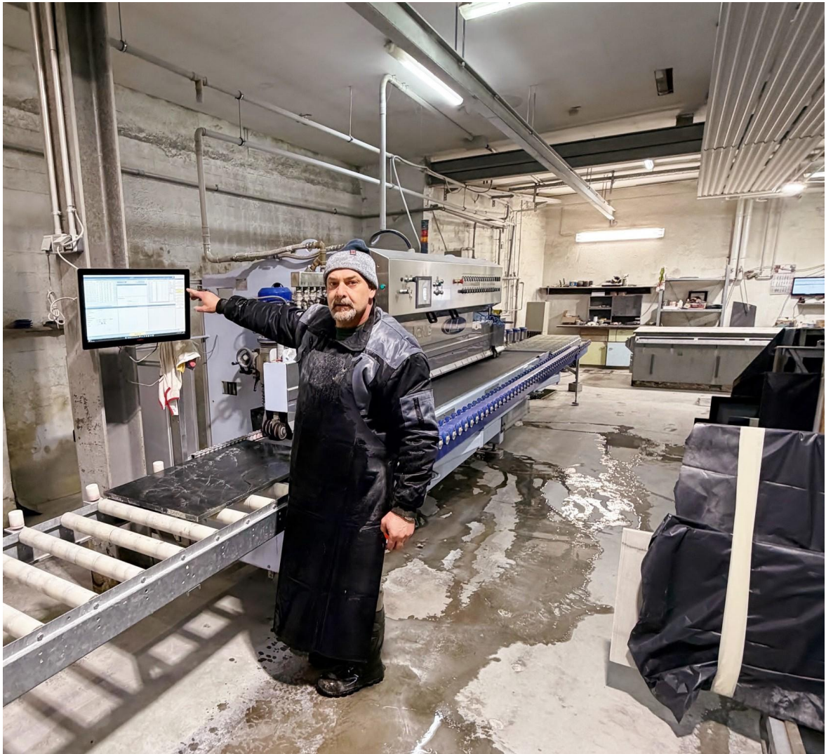
All machine and manual stations are equipped with their own PDA terminal (Production Data Acquisition Screen), featuring interfaces for data input and recording – including the Montresor edge polishing machine.
